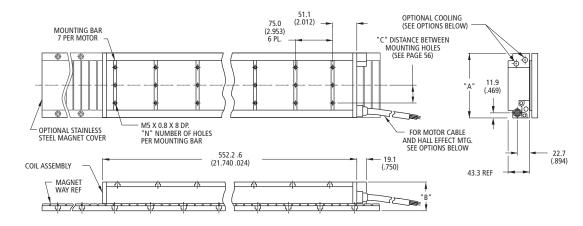
Resultant airgap = 0.9mm (.036) nominal (0.5mm (.020") minimum) when components are set up to dimension "B" in table below. (Please refer to installation manual for more detail)
