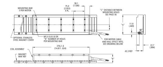
Resultant airgap = 0.9mm (.036) nominal (0.5mm (.020") minimum) when components are set up to dimension "B in table below. (Please refer to installation manual for more detail)
