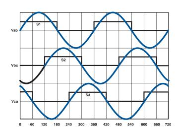
• Motor BEMF phases A,B,C relative to Hall effect devices \$1,\$2,\$3 with coil travel direction towards the motor output cable assembly exit as shown below.
