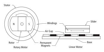
Rotary Motor Rolled Out Flat
