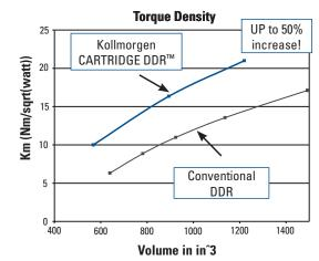
Proprietary electromagnetic design gives CARTRIDGE DDR<sup>™</sup> motors more torque per volume than conventional DDR technology.
