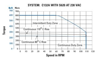
Notes: 1. At 40°C Ambient. 2. Increase Tc by 1.06 times for 25°C Ambient. 3. Temperature rise assumes a 20 x 20 x 0.75 inch Aluminum mounting plate or equivalent.
