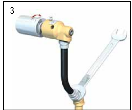
3 Connect flexible hose to supply line.
