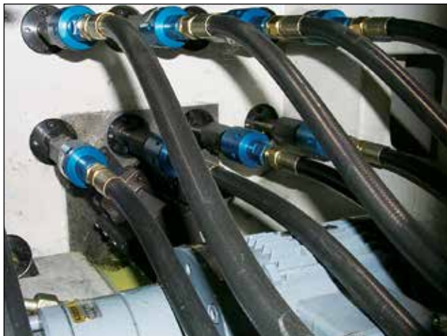
DEUBLIN 1116 Bearing-Supported Unions on Automotive Transfer Line
