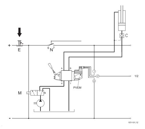
The difference between this safety method and the one previously described (1) is that here there is no built-in automatic fault monitoring and a neutral position switch (N) is connected.
