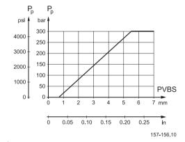
exceeds the load pressure before the working function is applied. If the main spool is held in this position, the pump pressure will remain constant – even if the load pressure changes – giving a stable system.
