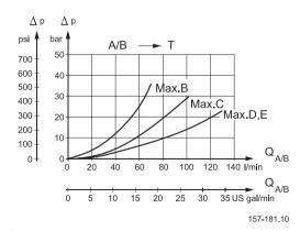
Spools D and E have the same opening area for forward flow and return flow. Spool E can give 100 l/min [26.4 US gal/min] pressure compensated oil flow due to a higher pressure drop across spool E.This occurs during spool actuation only.
