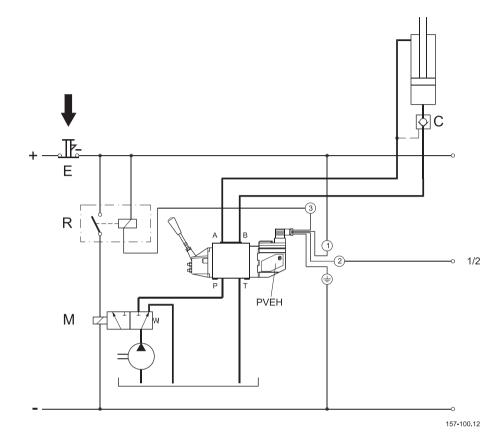
When the fault monitoring system in PVEH is connected, the reaction to electrical and mechanical faults (e.g. a spool seizure) is fast and operator-independent. See page 23 "fault monitoring".
