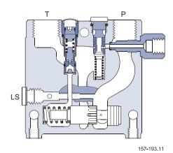
When the main pump flow fails, the external shuttle valve ensures that the oil flow from the manually operated emergency pump is used to pilot open the over centre valve and lower the load. The load can only be lowered using the mechanical operating lever of the PVG 32 valve.
