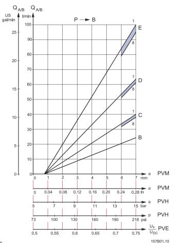
U<sub>S</sub> = Signal voltage U<sub>DC</sub> = Supply voltage 1 = First PVB after PVP 8 = Eighth PVB after PVP
