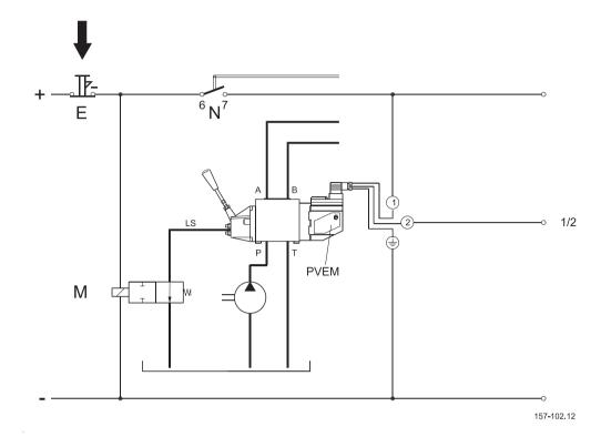
The difference from the previous method is that the LS- signal from the proportional valve is led direct to tank when the emergency switch (E) is actuated. This can be achieved by using the Sauer-Danfoss LS unloading valve PVPX, integrated in the pump side module.
