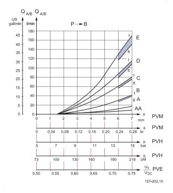
The oil flow is dependent on the pressure difference between the pump pressure and the LS signal. Normally the pressure difference is set at the LS pump regulator.
