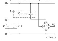
A: External relay B: Solenoid valve (e.g. PVPX)
