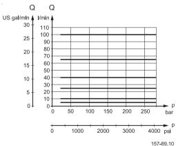
Oil flow at LS pressure limiting, pressure-, compensated PVB
