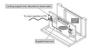
Connection to [CN12] on Oil Cooling Unit control board via supplied lead wire.
