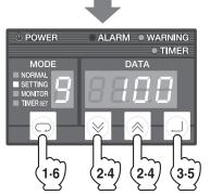
Example) Capacity direct designation (Capacity setting: 100%)
