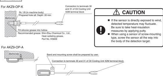
Place the thermistor in contact with the machine body, and cover it with putty.
