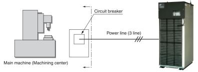
Starting/stopping the Oil Cooling Unit with the remote control contact (see page (10)) When the remote control switch is turned ON, the Oil Cooling Unit starts operation. To stop the unit, turn OFF the remote control switch.
