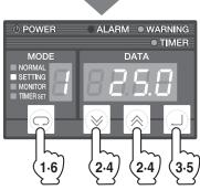
Example) Outlet oil temperature, Fixed temperature control (Temperature setting: 25°C)
