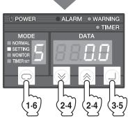
Example) Outlet oil temperature, Room temperature tuning control (Temperature difference setting: 0.0°C)
