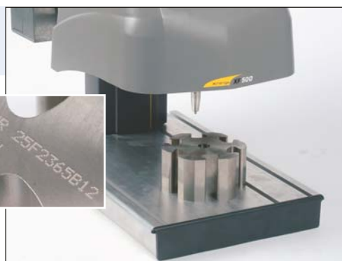
Marking DataMatrix™ codes in aeronautics subcontracting
