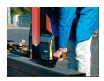
Marking of bulky parts (beams, tanks, vats, trailers).
