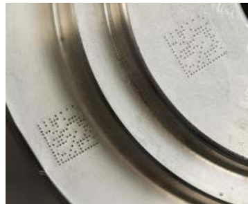
Marking on inclined plane, distorted surface, uneven flatness
