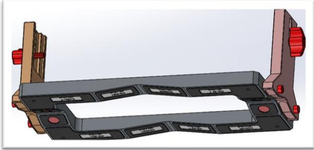
Part Number :- HD4614 Aluminium Front Fixture with V Groove & Permanent Magnets
