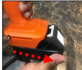
Step 3: Put base of machine handle on battery as shown in image.
