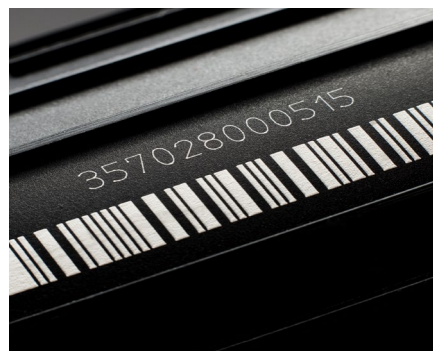
Contrasted marking on plastic
