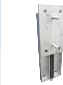
Back plate for 450 mm buffer 720 x 250 x 66 mm Weight: 32 kg Spring loaded. Follows the truck when loading.
