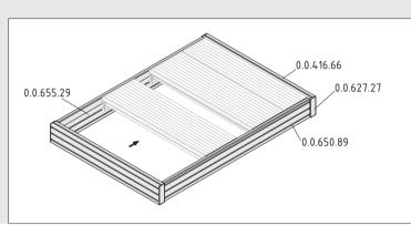
The basic frame that accommodates the floor surface consists primarily of Frame Profile 8 120x40 light, which is joined via its end-face to Profile 8 120x40 light.
