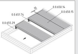
The panels can either be arranged to form one solid surface or be installed with 10-mm gaps between them. Platform Cleats produce a consistent gap that allows liquids to drain away, for example. Unbroken surfaces with no hazardous edges to present a trip hazard can be built using Angle Brackets 8 40x40x40 St and Step Spacer Profiles 24x8.
