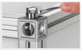
Threads need to be tapped into the core bores of the profiles that are being connected together with item cube fasteners. You can request profiles that come with these threads already tapped by ordering the service "Connection Processing, End Face, Thread M8x18" (0.0.026.95).
