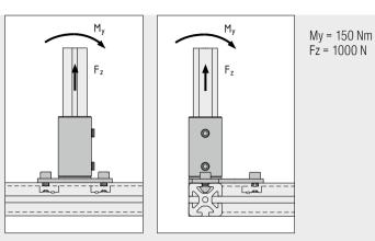
**Note:** In addition to the maximum load-carrying capacity of the Flange, it is important to take into account the load limits of the adjacent components in the construction.
