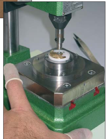
Zoom on the marking operation of the watch component
