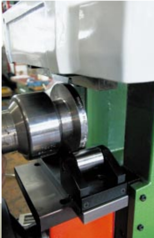
High pressure valve body marked on a MB 71EP
