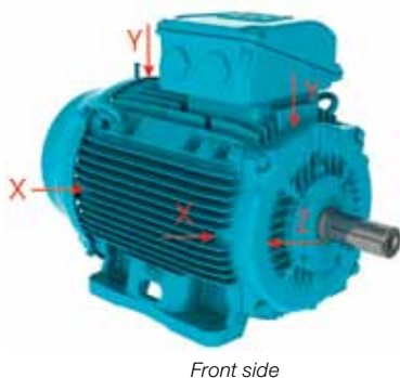
Figure 6 - Flat surfaces for vibration monitoring on the back and front side
