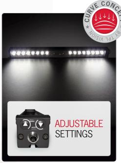
The EBAR Curve is a high power LED solution. It has been developed to ease the integration process and helps you achieve the best balance between brightness and homogeneity. The curve effect works by reducing the saturated light spot in the centre of a cameras Field of View (FoV). By reducing this spot, uniform illumination across the FoV can be achieved. This new development in machine vision illumination allows for smaller barlights to be used, giving you savings spatially and economically.
