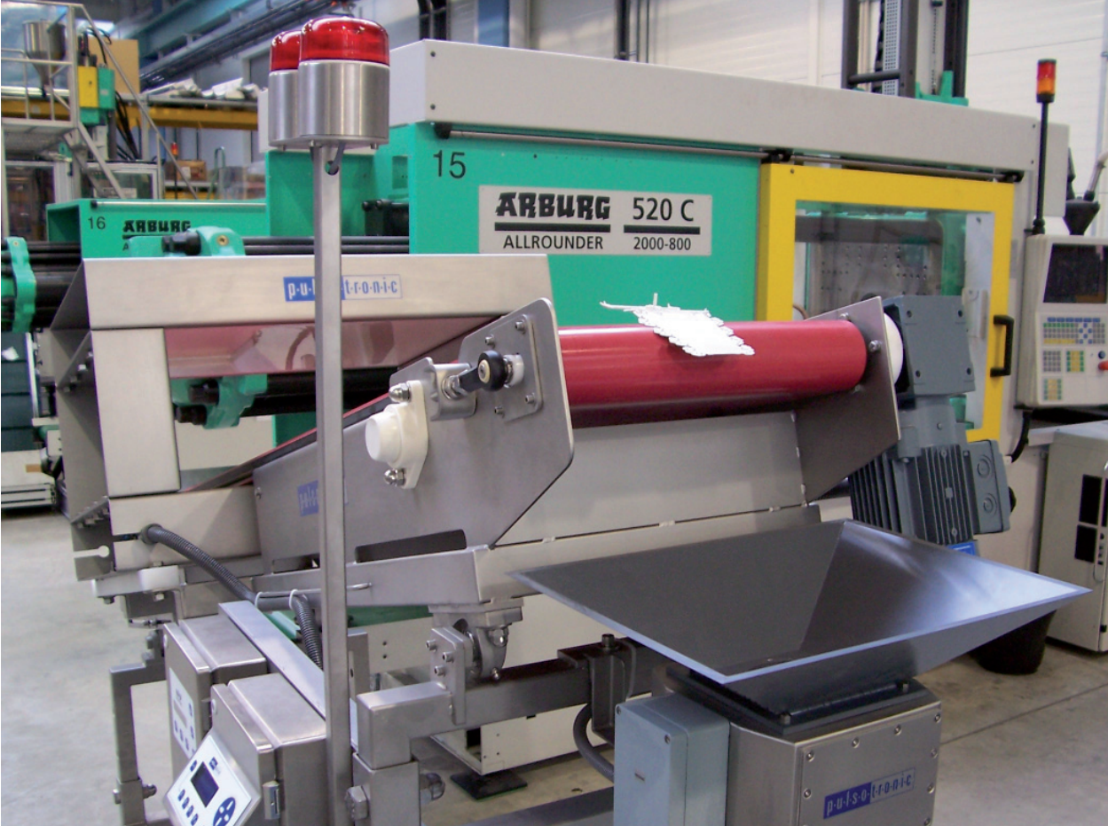
The Digital+ KS 100 for controlling nuclear fragments on downstream conveyor belts to injection moulding machines. (Illustration showing upstream tunnel detector)
