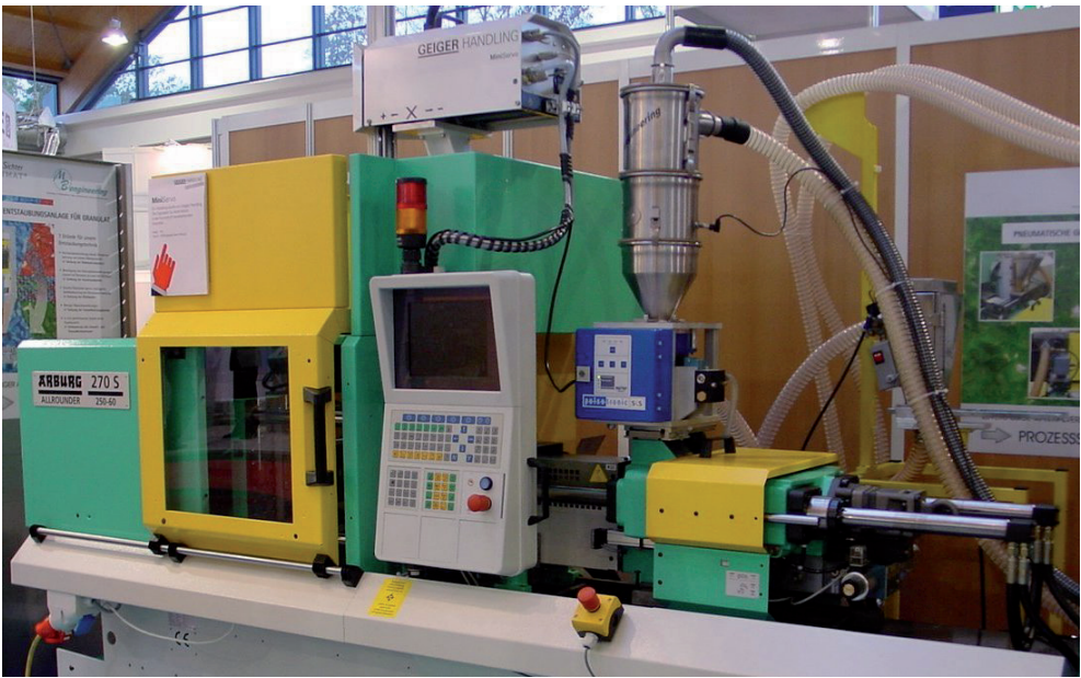
Digital Compact 50 directly mounted on an injection moulding machine.
