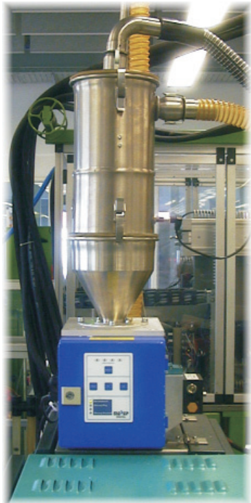
Digital Compact 50 for control of plastic granulate with mounted silo and vacuum conveying plant.
