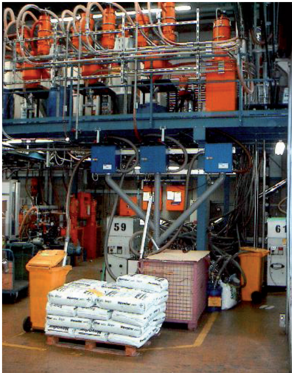
Three MESEP Extractor 70 provide for metal-free products.
