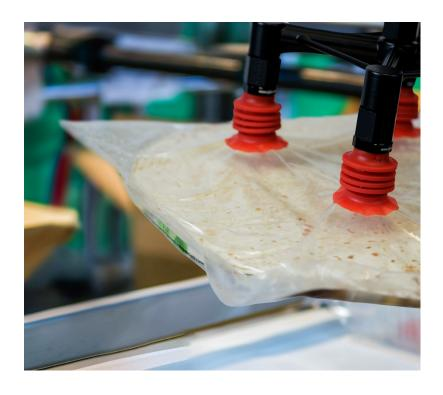
The BL-4 cup is designed for bags with fragile content such as snacks or frozen food. To suit this application, it is equipped with a longer lip and cleats.
