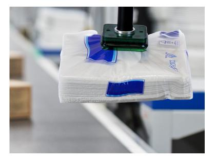
RBL cups are Piab's family of rectangular and square bellows cups, all configurable with many fitting options. Originally developed for flow-pack packaging machines, RBL cups are handy for lifting thin paper bags or bags made of slip sheets or plastic film.
