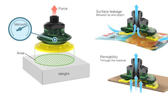
In many automated handling applications, vacuum and suction cups grip and move the bags. Different characteristics of the bag require different bag handling solutions. With the knowledge of vacuum technology and gripping solutions, Piab offers one of the market's widest ranges of suction cups so that each application will have a suitable solution.
