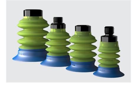
**Piab's BGI bag lips** from the configurable piGRIP® family provide a good grip on many different bags. Made in a durable and FDA & EU approved material, they are the perfect choice for lifting both sturdy plastic bags and stand-up pouches filled with dry or wet food/substances and liquids. The enhanced BGI-2 lips also provide an improved grip on thin, flimsy, and fragile plastic bags.
