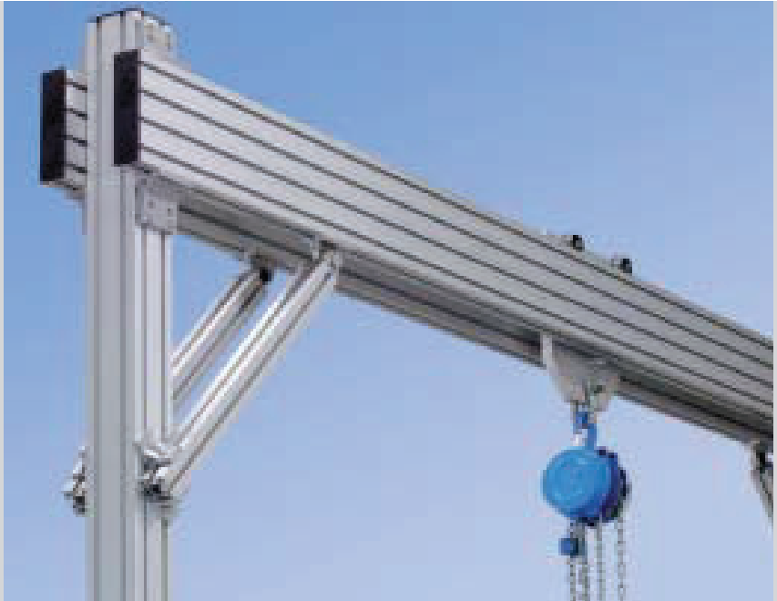
Mobile gantry crane made from series 50 profiles, span 3000 mm, max frame load 1000 kg, max deflection < 2 mm
