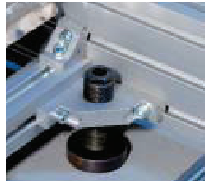
Leveling pad for subsequent anchoring to the floor
