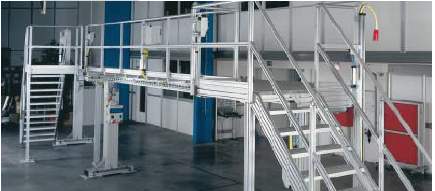
mk platform with stairs made using mk 2040.68 profiles
