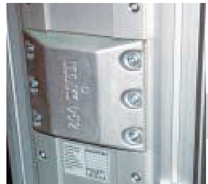
Cross-bracing using an mk connecting console
