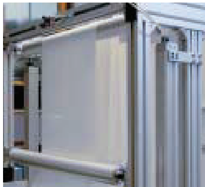
Film storage with pneumatic linear drive
