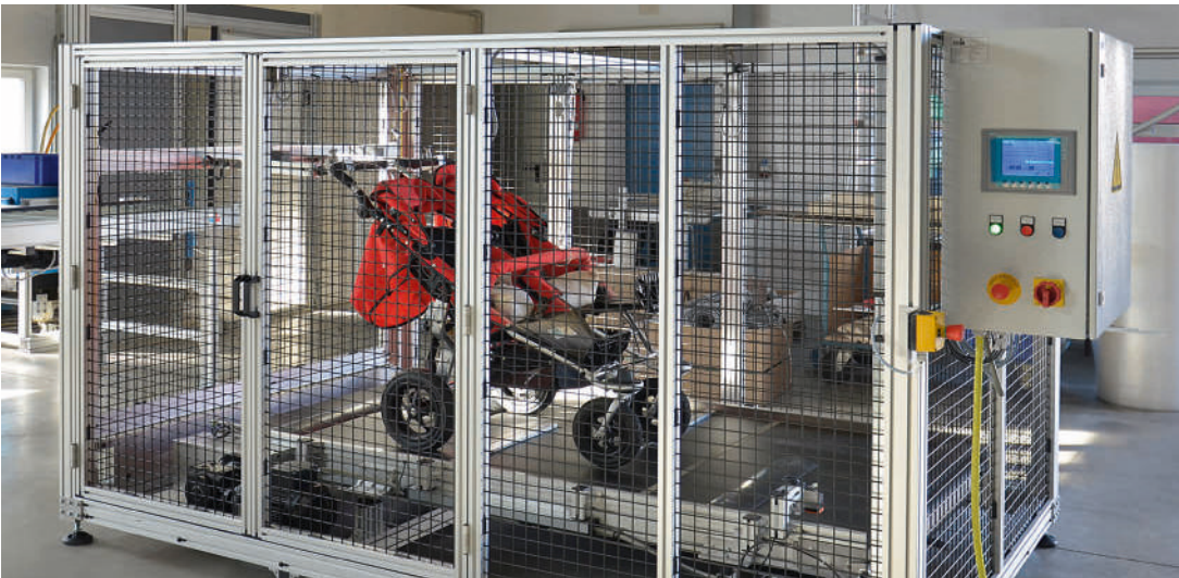
Custom guarding for pushchair test bench
