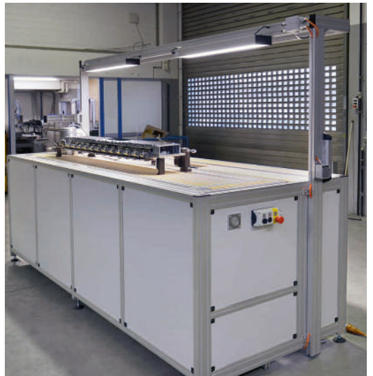
Assembly workstation with lowering mechanism based on electrically driven hydraulic cylinders
