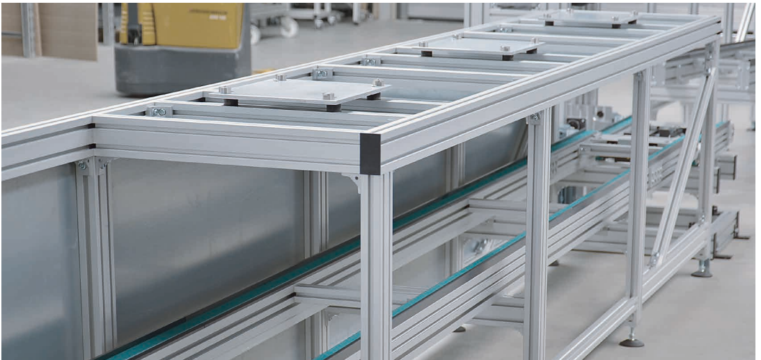
Base frame with levelling feet and holders for workpiece carriers
