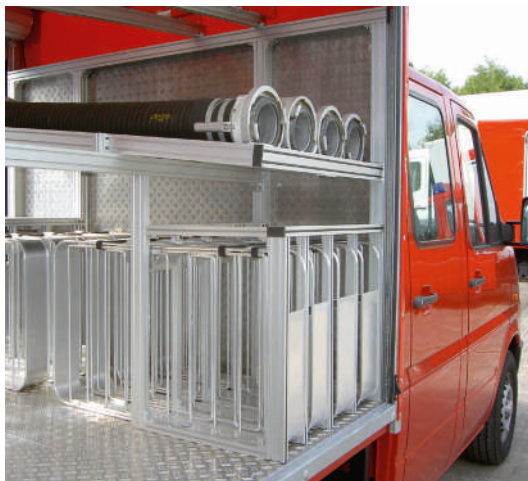
Fire engine interior built from Series 25 profiles
