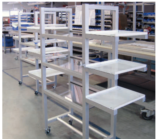
Material supply trolleys made from Series 40 cleanroom profiles with acrylic shelves
