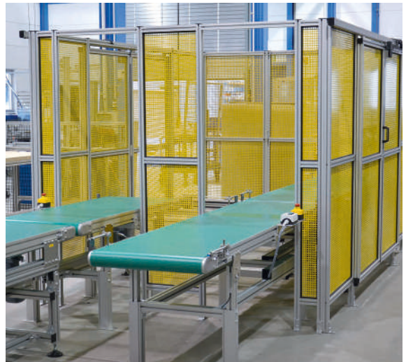
Custom protective device guard made from partitions with powder-coated perforated sheets and sliding doors with solenoid latches
