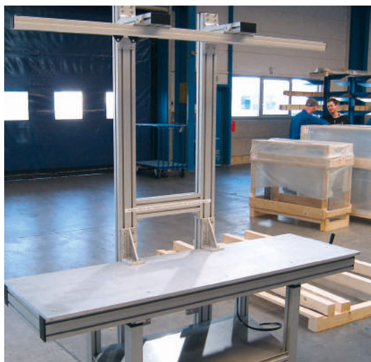
Assembly workstation with crank-operated manual height adjustment, 600 kg load capacity
