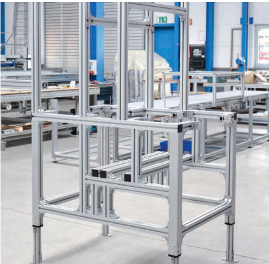
Machine frame made from Series 50 profiles
