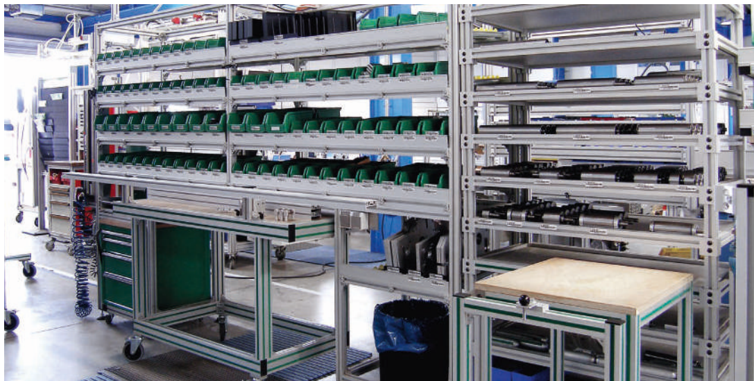
Kanban workstation for increasing productivity by decoupling assembly and supply logistics
