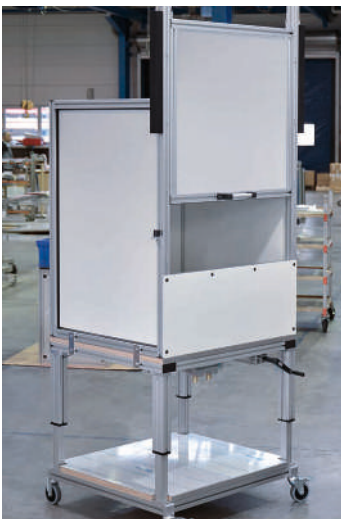
Workstation with protective cover and manually adjustable sliding element
