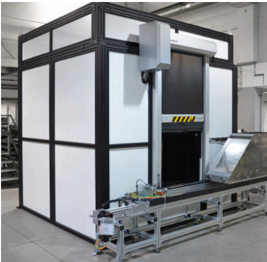
Measuring chamber made of black anodised profiles with automated feed and removal
