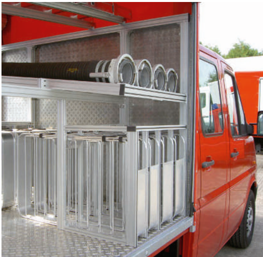
Fire engine interior built from Series 25 profiles
