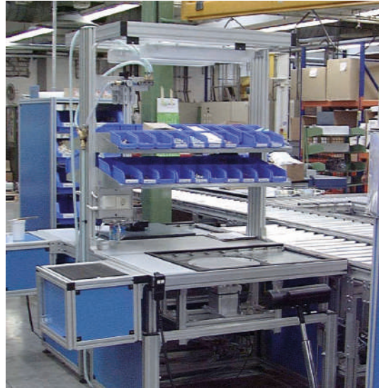
Industrial workstation in DFT flow line for manufacturing vacuum pumps
