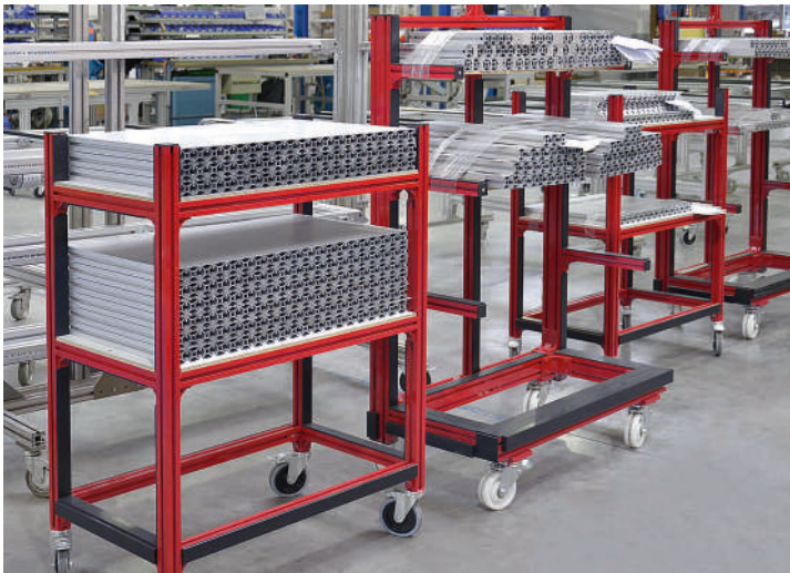
Supply trolley made from Series 40 profiles painted red
