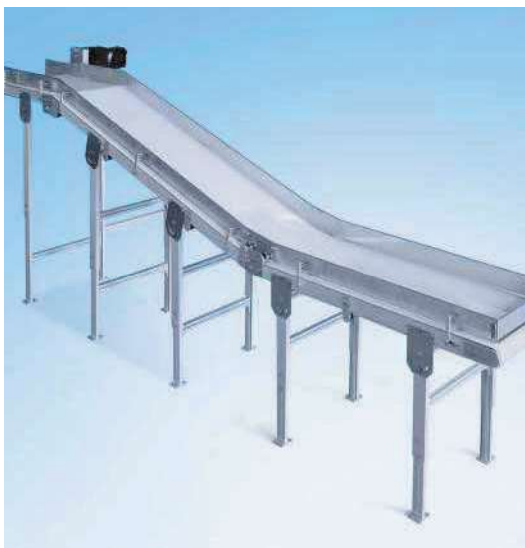
Incline conveyor belt KFG-P 2000 with head drive AC and side rail, belt guide via longitudinal cleats K10
