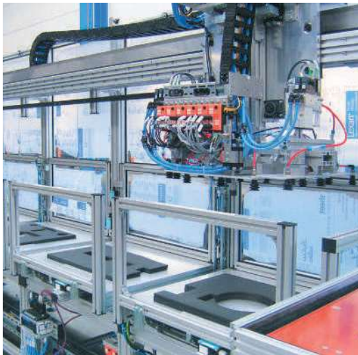
X-Z gantry with additional pneumatic weight balancing as a holder for a vacuum gripping system
