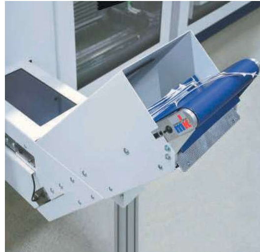
Belt conveyor with low installation height integrated into blister packing system
