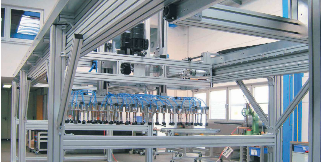
Two-dimensional gantry with vacuum gripper as a handling and loading system for steel. Two independent loading systems on a common X axis with gear rack with track rollers and riding rack drive
