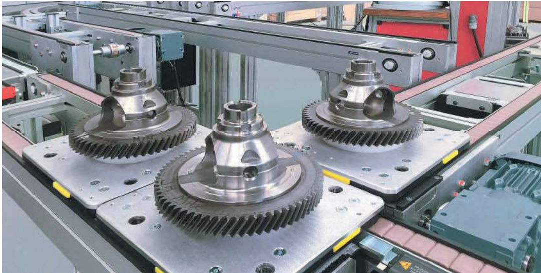
Versamove standard with flat top chain conveyor and lift-and-transfer conveyors
