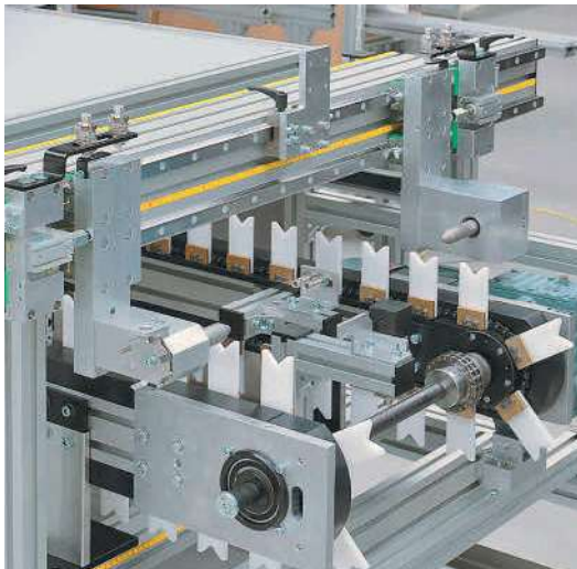
TKU 2040 for transporting camshafts with positioning sensors
