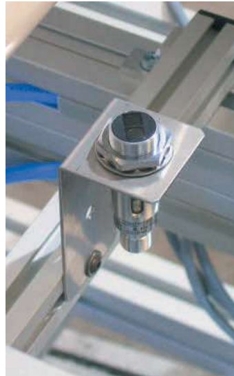
Initiator holder made from VA steel sheet
