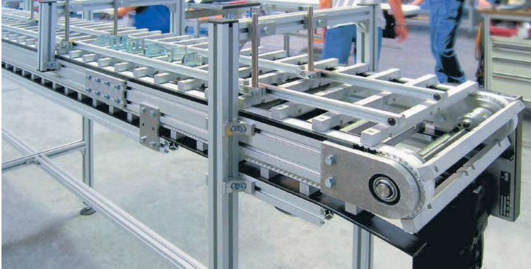
ZRF-P 2040, threaded sleeves integrated into the timing belt enable customer-specific cams to be bolted on
