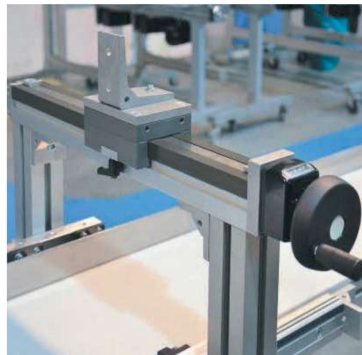
Manual two-axis adjustment system for holding a marking device with VST 2015
