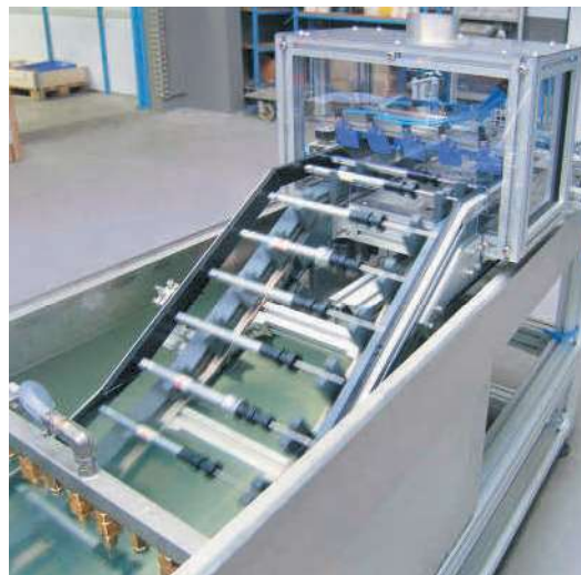
TKU 2040 with 20° inclination and transport of workpieces through a cleansing bath
