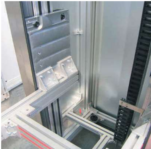
Double-LZR 2005-38.44-30 with side mounted carriage plate and cantilever for conveyor as lift
