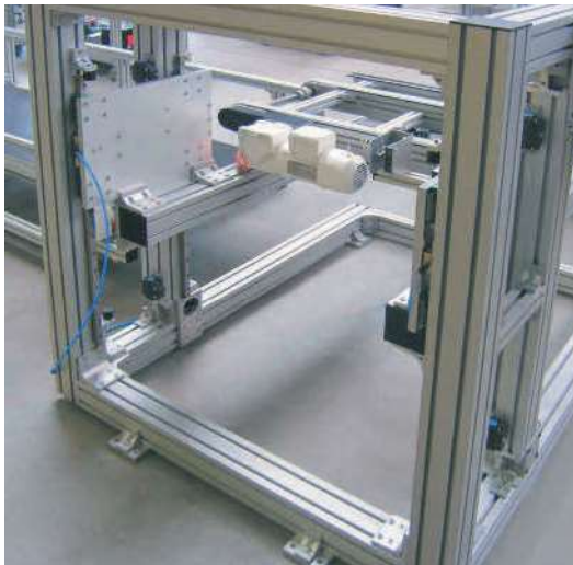
Lifting unit with LZR with recirculating ball bearing guide KU 25 with profile cantilever for supporting the ZRF-P 2010 conveyor
