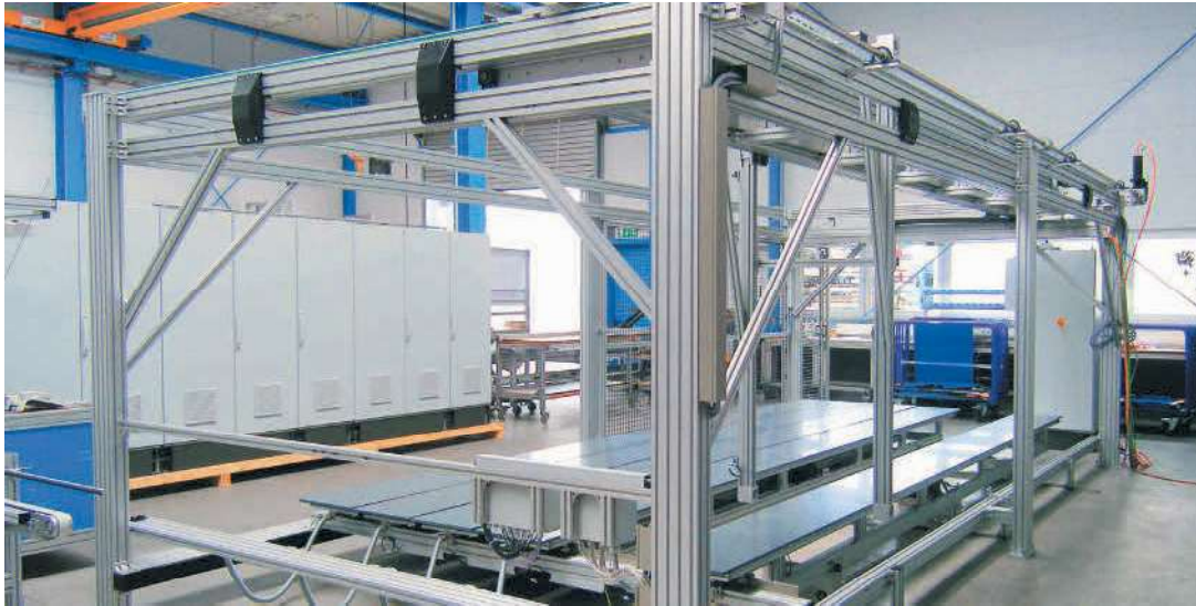
X-Y-Z handling gantry for regular monitoring of plant growth
