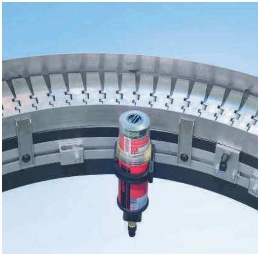
Special flat top chain conveyor with a width of 205 mm with side rail SF 2.1 and lubrication station
