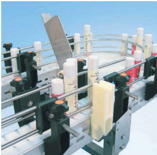
Interlink with INOX flat top chain conveyor with rolling 180° curve
