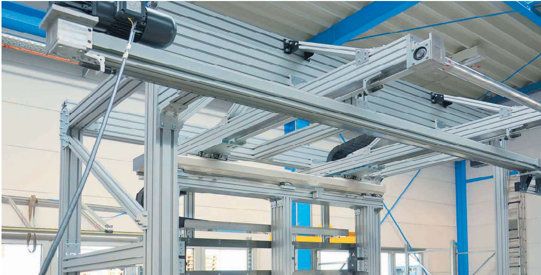
Two-axis gantry for handling sleeves with parallel gripper
