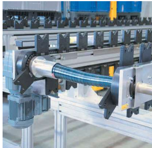
TKU 2040 for transporting camshafts with a spiralled cover as a protective guard on the connecting shaft
