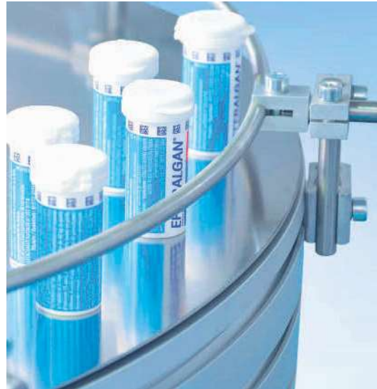
Rotary table DT-P 2040 with side rail, similar to SF01
