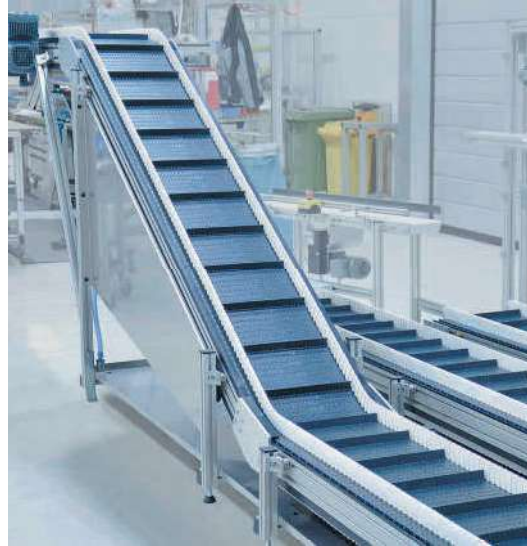
Incline conveyor KFM-P 2040 with white side plates and drip pan
