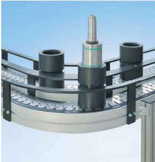
Double-line flat top chain conveyor SBF-P 2254 with sliding 90° curve and individual side rail
