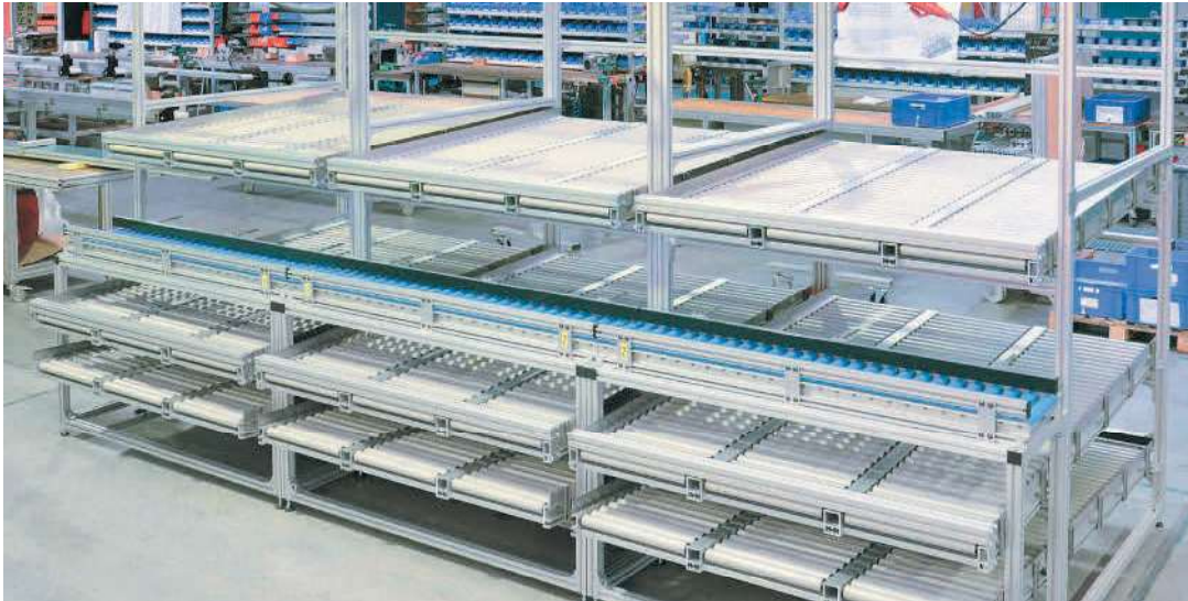
Kanban workstation with RBS-P 2065 gravity conveyors for feeding products
