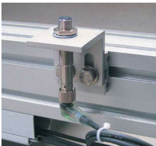
Initiator holder made from aluminium angle bracket
