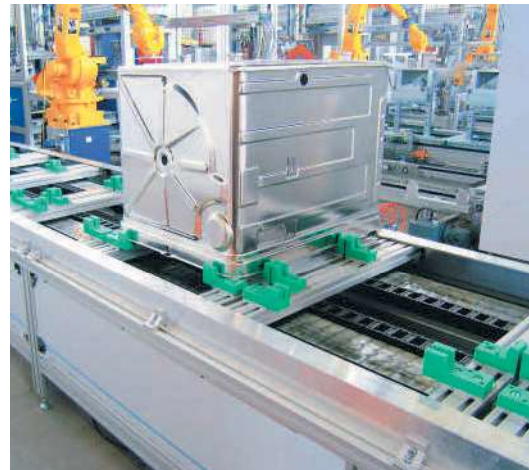
SPU double-line as an infeed conveyor for dishwasher housings
