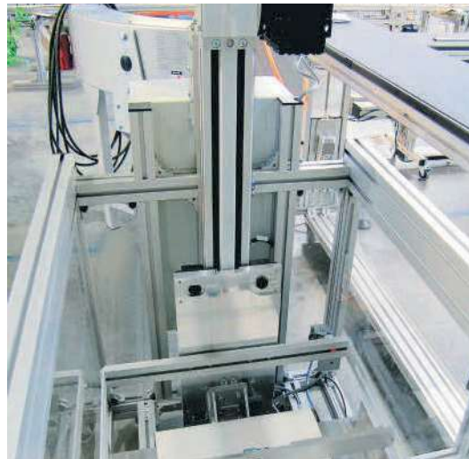
Linear module type LZR 2005-38.44-30 with motor and controller as a lift with a belt conveyor
