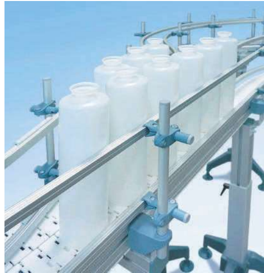
Versaflex SBF A08 with height and width-adjustable side rail
