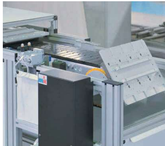
Single-line SPU with custom pallet holder
