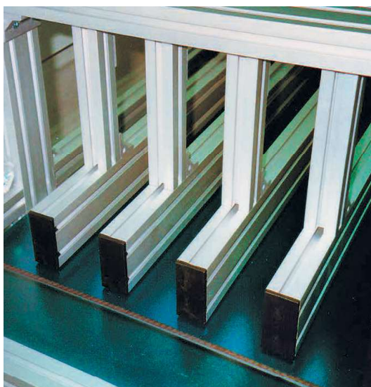
Multi-line, adjustable side rail in gantry arrangement
