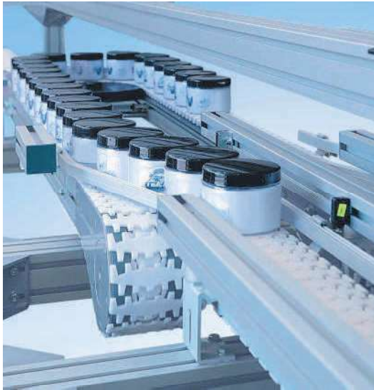
SBF Versaflex with adjustable side rails
