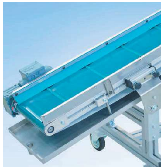
Belt conveyor GUF-P 2000 AF as inclined conveyor with cleats, special side rail and drip pan
