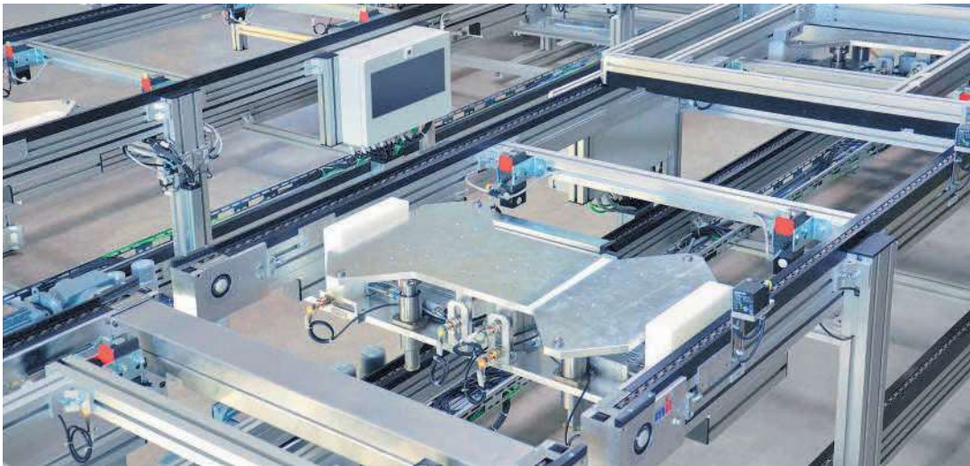
Versamove plus with accumulating roller chain conveyor SRF-P 2010 AF
