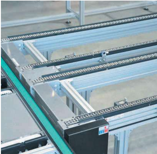
Dual-lane KTF-P 2010 with 80° C temperature resistance
