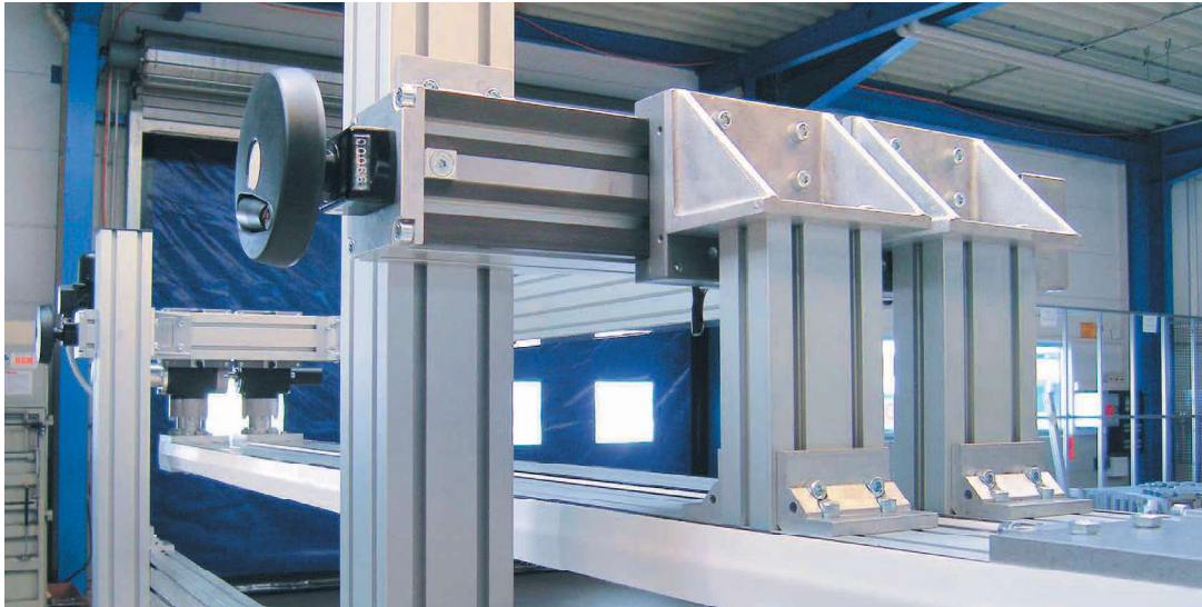
Dual VST 2011 for manual lane width adjustment on a side conveyor
