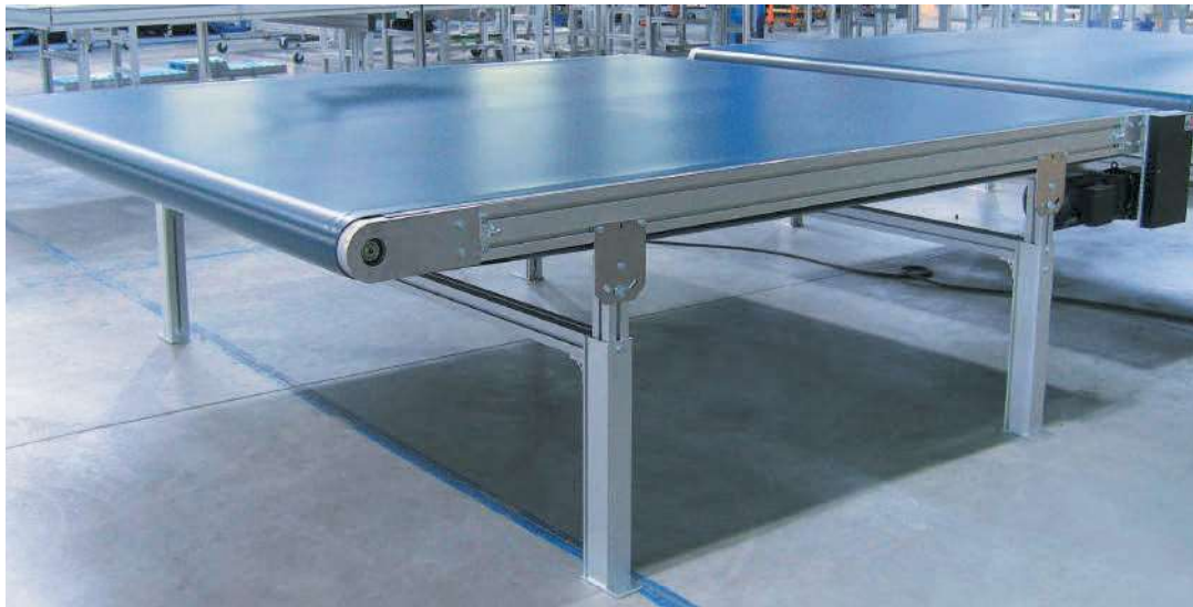
GUF-P 2004 designed with maximum width B=2 m
