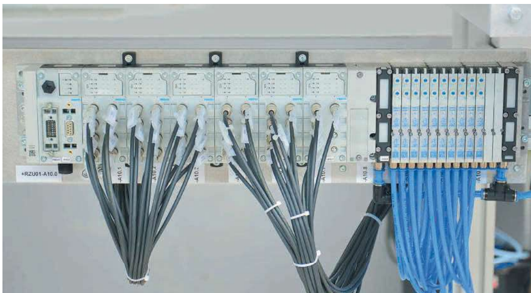
Valve terminal with input and output module
