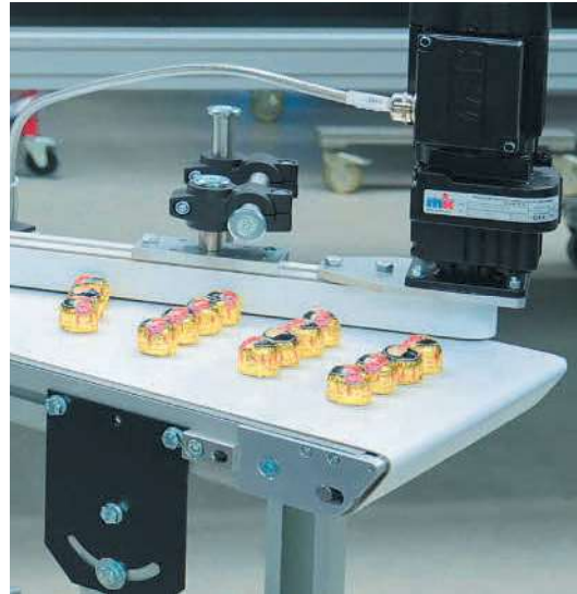
GUF-P 2000 with rolling knife edge and separator conveyor with head drive AF
