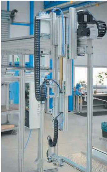
Gantry stand with telescopic gripper unit
