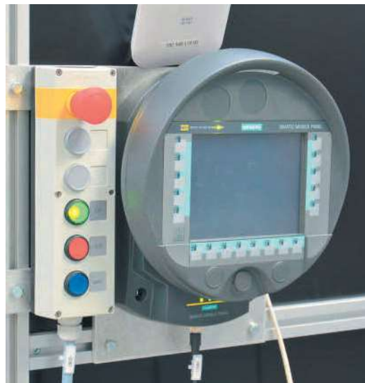
Door dial with emergency stop button and mobile operator panel
