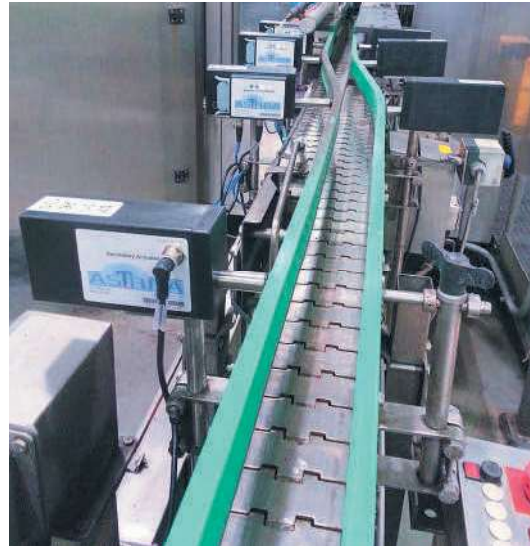
Versaflex SBF stainless steel conveyor with automatically adjustable side rail ASTRRA
