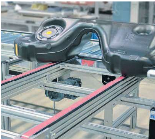
Interlink ZRF-P 2010 as discharge line for fuel tank
