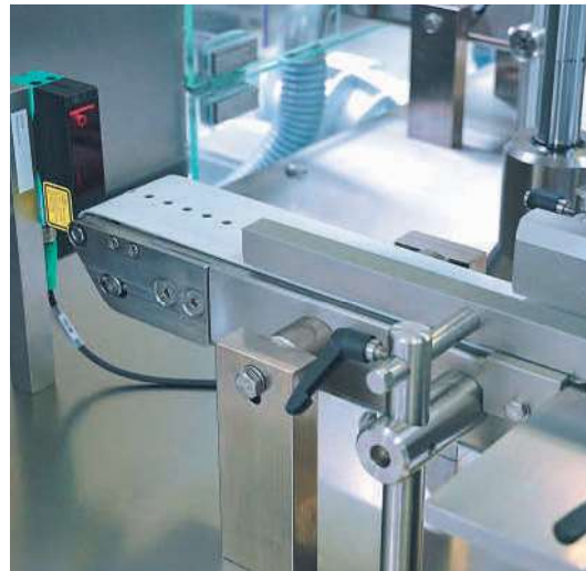
INOX vacuum belt conveyor with custom side rail
