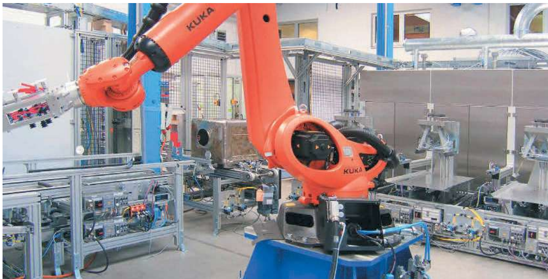
Turnkey interlink system, including controller and protective device guard with integrated robot island and melting ovens
