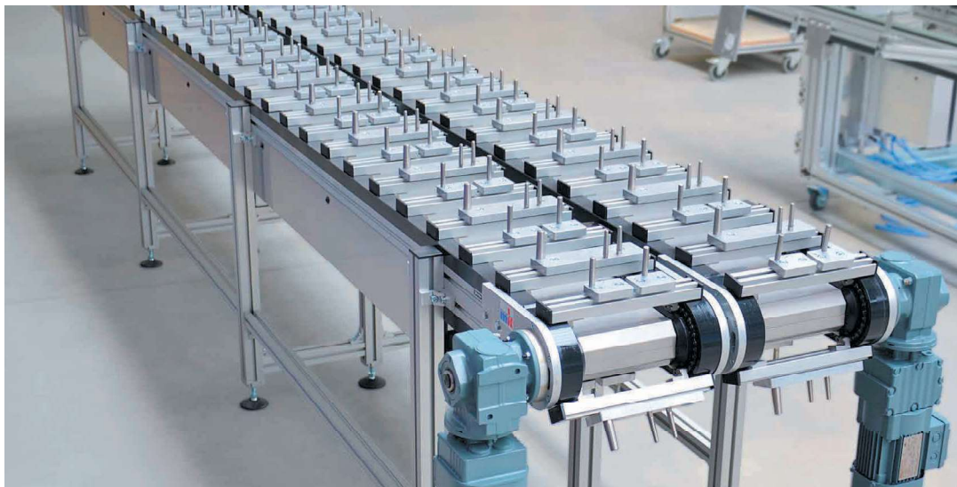
TKU as dual-line system with custom profile pallets and holders
