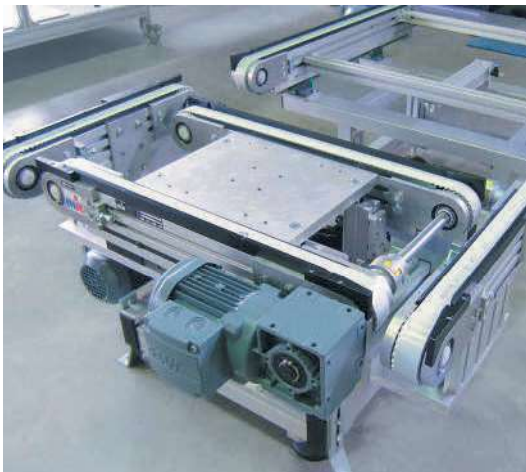
Lift and transfer with turn station and pneumatic feed stroke
