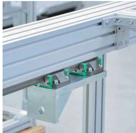
Frame for stress testing based on KU 30.10 recirculating ball bearing guide
