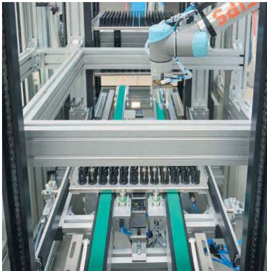
The pallet is transported in and out of a production cell through a double-line timing belt conveyor
