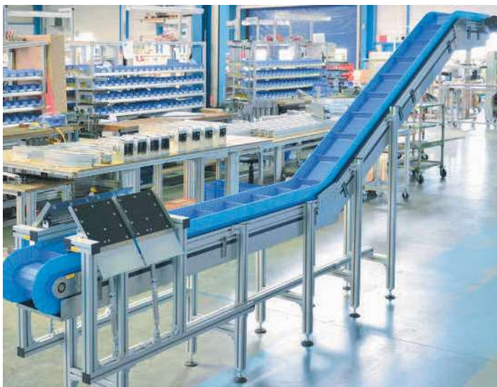
KFM-P 2040 with drip pan and separator flap
