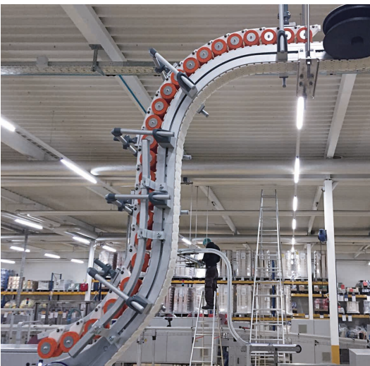
Versaflex flat top chain conveyor with guide rollers for vertical transport
