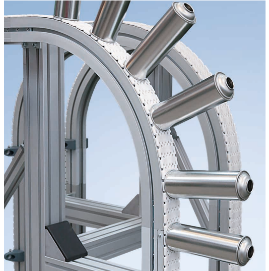
Versaflex SBF A08 with magnetic chain for vertical transport
