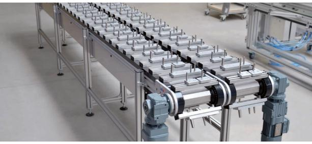
Double-conveyor system with order-specific profile pallets and fixtures
