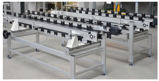
TKU 2040 with special adjustment unit for adjusting the distance between the chains
