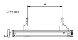
You can adjust the position of the non-driven chain by turning the handwheel, which lets you conveniently vary the distance between the chains. A digital gauge shows the displacement.
