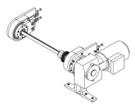
The adjustable drive has a special shaft with a ball bushing that lets you easily adjust the width. The motor's torque arm has a bracket for attachment to a sturdy base frame.
