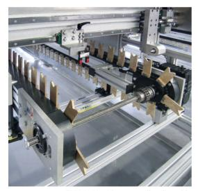
TKU 2040 with a manually adjustable chain and a lifting/turning unit
