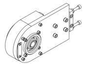
Tail 19 has the same design as tail 01. However, it is equipped with a Ø 20H7 hollow shaft that can be attached to an insert shaft with a feather key for coupling drives or for connecting a rotary encoder. It can be used in conveyors with both fixed and adjustable widths.
