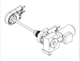
The drive is dimensioned according to the specified conveyor width. The torque arm has a bracket for attachment to a lighter stand system.
