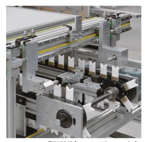
TKU 2040 for transporting camshafts with positioning sensors
