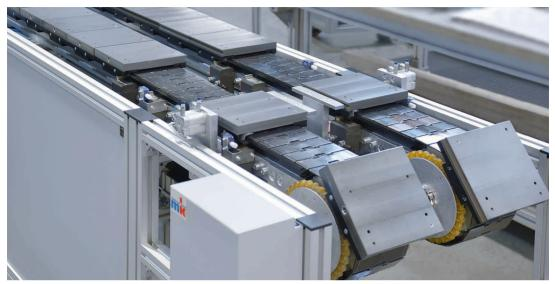
SPU 2040, dual-line, 114 chain width with positioning unit
