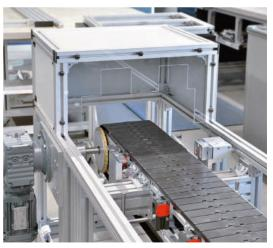
SPU 2040, single line with protective device guard with pendulum flap
