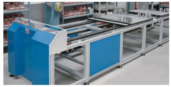
SPU 2040, double-line with separating function for supplying parts in an assembly and welding facility
