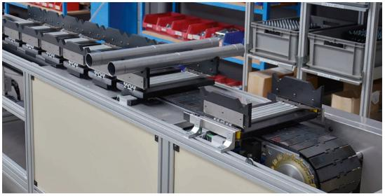
SPU 2040, single line with pallet separating function for supplying parts in a production facility
