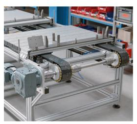
SPU 2040, double-line, 114 chain width with customer-specific pallet
