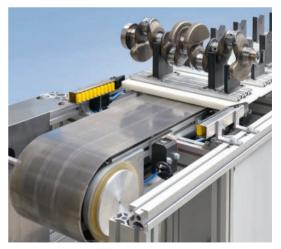
SPU 2040, single line with special chain and lateral positioning via roller strips
