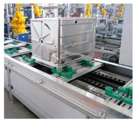
SPU 2040, double-line as infeed conveyor for dishwasher units
