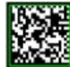
Quiet zone violation
