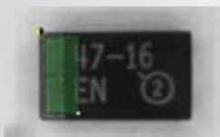
Capacitor Oriented Correctly
