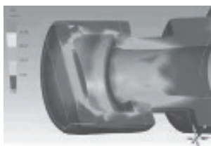
Simulation (FEM method) of the stress distribution under high pressure on housing and ceramic cap
