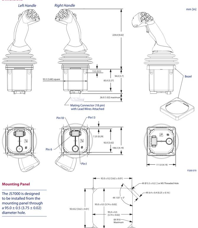
The mounting flange of the JS7000 should be connected to the vehicle chassis ground.
