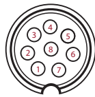
DP600 Binder Series 702 USB Connector 3 pin out information
